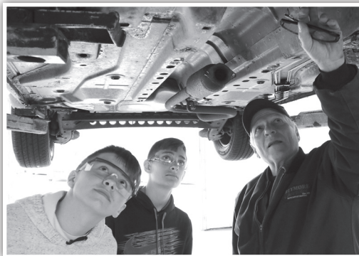
After reviewing safety procedures, Tom Bozzuto of Reymore Chevrolet shows CSMS students John Snyder IV and Dylan Brown how to replace an exhaust system.
